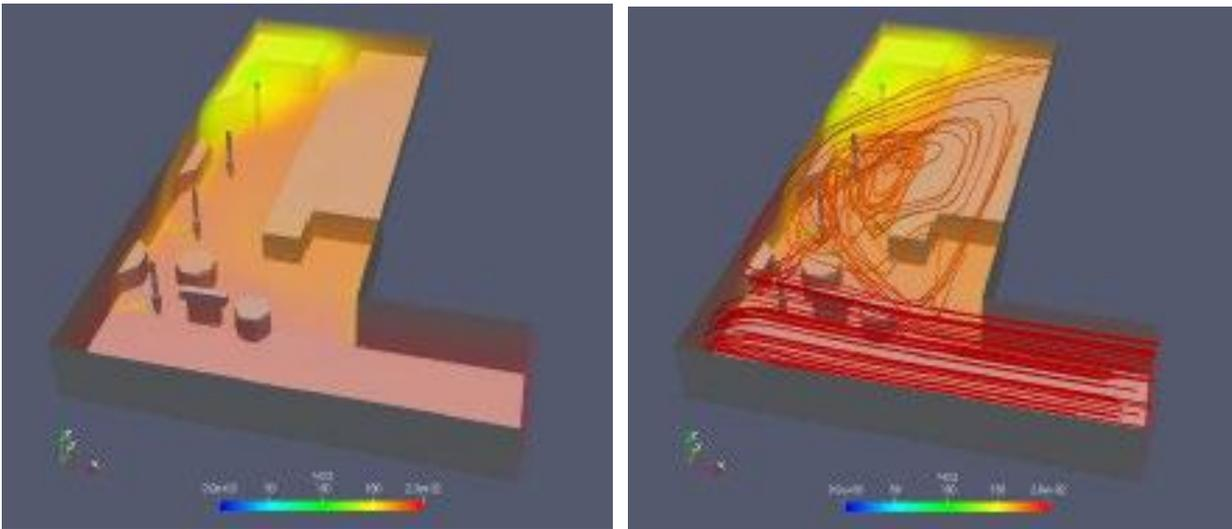
Figure 4. CFD simulations of airflow and  $\text{NO}_2$  levels in Marylebone Station:  $\text{NO}_2$  concentration (left); airflow streamlines and  $\text{NO}_2$  concentration (right).
