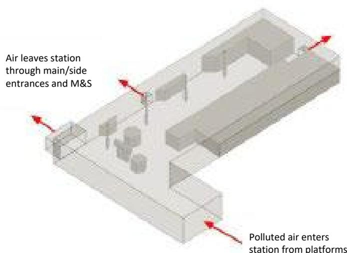
Figure 3. The CAD model of Marylebone Station, showing the locations of the four cylindrical advertising casings with AirBeams installed. The polluted air enters the station from the platforms and exits through several openings.
